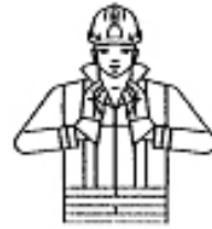
Indicating horizontal distance
